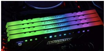
The modules feature 16 RGB LEDs per module, as divided in 8 zones. To further add customisation, customers can remove the light bar and 3D print own designs. Other features from the Tactical series are present, such as XMP profiles, black PCB and custom heat spreaders.
