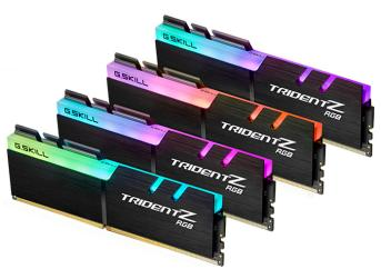
G.Skill follows on the launch of the Intel Z390 chipset with a pair of high-performance Trident Z RGB dual-channel memory kits-- a 16GB (2×8 GB) kit rated for DDR4-4800 CL19 22-22-42, and a 32GB (4×8 GB) kit rated at DDR4-4500 CL19 22-22-42.
