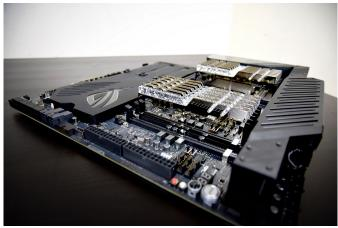
The 6-channel memory kits promise XMP 2.0 supported speeds of up to DDR4-4000 CL17-18-18-38 at 1.35V, thanks to Samsung B-die memory ICs. They range in rated frequency from 3200 to 4000MHz, and in size from 4GB (8GB x6) to 192GB (16GB x12). According to the company, the DDR4-4000 CL17 96GB (8GBx12) kit offers real bandwidth of 122GB/s, a "substantial incease" compared to currently available quad-channel platforms.
