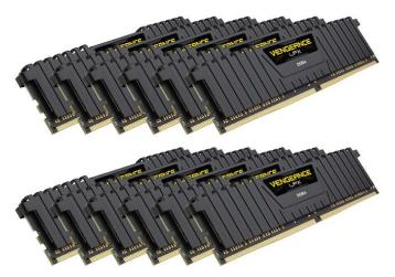
The 96GB kit (CMK96GX4M12P4000C19) offers DDR4-4000MHz speeds, with 19-23-23-45 timings at 1.35V, and consists of twelve 8GB sticks. Meanwhile the four 192GB kits are based on speeds, specifically DDR4-2666, DDR4-3200, DDR4-3600, and DDR4-4000. Each kit consists of twelve 16GB sticks operating in hexa-channel mode on the Xeon W-3175X and other LGA3647 CPUs allowing for UDIMM operation. The DDR4-2666 option operates at 1.2V, while the others require 1.35V.
