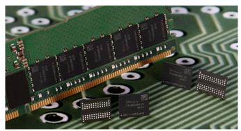
As detailed by EETimes, the chip runs at 1.1V and measures 76.22mm2. The presentation had the company describe the challenges of making the chip, such as the implementation of a modified delay-locked loop (DLL) using phase rotator and an injection locked oscillator to reduce the clock jitter and clock duty cycle distortion associated with operating at higher clock speeds.
