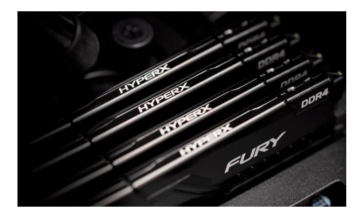
Based on 16Gb memory chips, the 32GB HyperX Fury unbuffered DIMMs and 32GB Impact unbuffered SO-DIMMS feature XMP SPD profiles for easier speed settings and are compatible with the lastest AMD and Intel platforms. The desktop-oriented 32GB Fury UDIMMs are rated for DDR4-2400/CL15 at 1.2V, DDR4-2666/CL16 at 1.2V, DDR4-3000/CL16 at 1.35V and at DDR4-3200/CL16 at 1.35V operation. The modules carry aluminum heat spreaders, and will be available solo, in 64B duos and in 128GB quartets.
