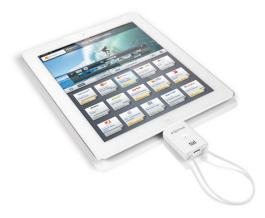
The Tizi Go is a follow-up on the Tizi, a wifi-based TV transmitter. Connecting to the iPad dock connector, it not only receives DVB-TV signals but also allows users to pause, record and rewind live TV via tizi.tv app.
