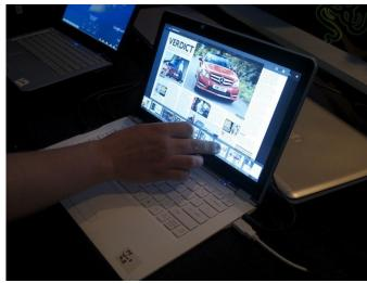
The touch-enabled ultrabook carries a capacitative display and is powered by a 1.5GHz lvy Bridge processor. Touch input works as well as any tablet, allowing one to easily navigate through the installed Zinio magazine app.
