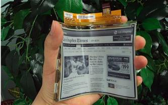
The LG design measures 6" diagonally and handles XGA (1024x768) resolutions. Construction is in plastic, meaning the display is only 0.7mm thick and weighs 14g (50% less than traditional glass displays). It is not able to handle colours or animation, but should offer a crisp reading experience.
