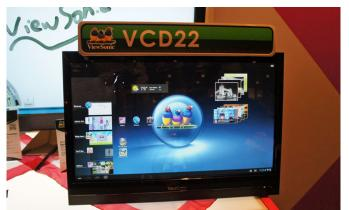
The VCD22 looks like an all-in-one desktop, but it carries a 1GHz dual-core TI OMAP processor and runs on Android 4.0. The 22-inch touchscreenhandles 1920x1080 resolution, even if it appears to suffer from low contrast and poor viewing angles.
