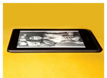
The display is a brighter version the one found in the Kindle Paperwhite, being a 300ppi number with a scratch-proof glass front. The display is micro-etched, which Amazon says helps light for glare-free reading and provides a paper-style feel.
