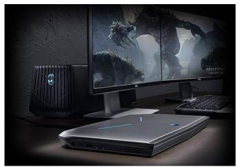
At 2.5cm thick, the Alienware 13 is the thinnest from the company, and as such it cannot carry the kind of hardware found in desktop gaming rigs. Enter the Graphics Amplifier, which houses full length, dual-height graphics cards such as the Nvidia GeForce GTX 600 series or AMD Radeon HD 5000 series. It connects to the Alienware 13 via proprietary USB/PCIe cable, and promises to push enough bandwidth to drive "desktop graphics experiences."
