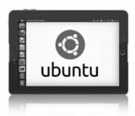
Hardware details include a quad-core 1.3GHz Atom Z3735D SoC, Intel HD Gen7 graphics, 2GB DDR3L RAM, 16GB storage, 2MP front/rear facing cameras and a 7900mAh battery. Connectivity comes through 802.11b/g/n wifi and Bluetooth, while the display handles 1280x800 resolution. The operating system is, of course, Ubuntu Touch, specifically the 14.10 release.
