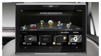
The Audi Tablet is a 10.1-inch Android number powered by Nvidia's Tegra 4 processor. Being designed specifically for automotive use it connects to the on-board infotainment and navigation system via CANBus and has a matte display designed to reduce both reflections and micro-vibrations passing through the car.
