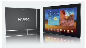
In order to avoid confusion, the "ARM" in the name has nothing to do with the chipmaker-- it actually stands for "Advanced Removable Modules." These are the CK PCB-HUB (connectivity options), CK Module (16GB flash storage), CK Core (Samsung Exynos 4412 quad-core processor, 2GB RAM) and the 10.1-inch 1280x800 touchscreen.
