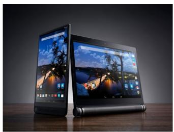
Like it smaller sibling, the Venue 10 features a 2560x1600 OLED display. It is powered by a quad-core Intel Atom Z3580 CPU, an RealSense depth camera and audio via MaxxAudio Mobile technology.
