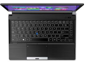
As well as the aforementioned Intel Mobile Performance processor, specifications include up to 16GB DDR3 memory and either 1TB hybrid HDD or 512GB SSD. Handling security are built-in Intel vPro technology, Trusted Platform Module (TPM) and a fingerprint reader, while connectivity includes three USB 3.0 ports, full-size HDMI, LAN port and media card reader.
