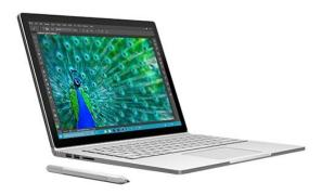
Described by the company as nothing less than a "redefinition" of the laptop, the Surface Book features a 13.5-inch optically bonded 3000x2000 resolution display users can remove for use as a regular tablet. One can also simply bend the flexible hinge holding the display to the keyboard all the way back for more support.
