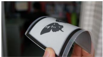
A long promised wonder material, graphene comes in layers just 0.335 nanometers thick. A conductor of heat and electricity, it allows for pliable ePaper displays with high-light transmittance. In addition, graphene ePaper is less expensive to produce, since the graphene involves cheaper carbon instead of the exotic indium metal required by regular ePaper.
