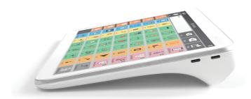
The Indi is a Windows 10-based device. It carries outward-facing speakers with "exceptional loud and clear" output, while control comes through either touchscreen, switch or head mouse. Included Snap software promises intuitive symbol-based communication, making it ideal for users with autism, cerebral palsy, Down syndrome and intellectual disabilities.
