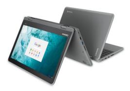
Allowing for the transformation between notebook and tablet modes is a 360-degree hinge, and one can also use the Flex 11 in 2 other modes, "watch" and "tent." Construction promises to be drop-resistant up to 75cm, while the keyboard can handle spills of up to 330ml, with channels draining liquid away from electrical components.
