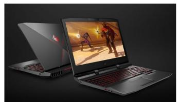
Being aimed at such high performance, the Omen X is a bulky machine. It comes in 15- and 17-inch options (with 4K or 120Hz 1080p display), weighs 5kg and packs high-performance fans and an integrated vapour chamber with four 3.5mm heat pipes pushing heat to four rear corner-mounted radiators. The result should ensure the GPU and CPU remain cool.
