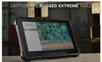
The Latitude 7212 has an 11.6-inch display and comes with either 6th or 7th generation Intel processors, 8/16GB RAM, from 128GB to 1TB storage and up to two separate 34Wh hot-swappable batteries offering up to 19 hours of use. It is also backwards compatible with docking solutions for desks and vehicles.
