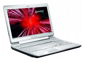
The F750 series uses the integrated webcam to track the user's eye position-- ensuring the 3D effect from the 15.6" display matches their viewing angle.
