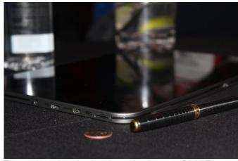
Powering the device is a dual-core OMAP 4430 1.2GHz CPU from Texas Instruments, while Bluetooth 2.1 and 802.11b/g/n wifi provide connectivity. Ports come in micro varieties of HDMI, USB 2.0 and SD card slot.
