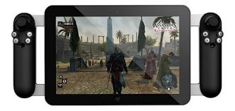
The prototype carries an Intel Core i7 processor, together with a 3-axis gyroscope, magnetometer, accelerometer and built-in force feedback. Connectivity comes through wifi and Bluetooth (Razer gives no mention of USB or HDMI ports), while Dolby Theatre v4 enchances audio.
