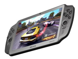
It runs on a dual-core 1.5GHz processor and a Mali 400mp quad-core GPU, and storage comes through 8GB internal and microSD card slot.
