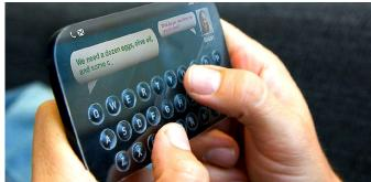
The technology inflates "tixels" (Tactile Pixels) at specific areas of the screen with small amounts of fluid, forming squishy, tactile buttons. Once the buttons are disabled the display returns to conventional touchscreen form.
