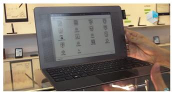
Like other hybrid devices, the Boox Typewriter consists of a tablet-style display and a detachable keyboard. The display is a 9.7-inch 1200 x 825 Carta elnk number, and handles touch input via either fingers or electromagnetic (EMR) stylus. It also carries a 1GHz Cortex A9 CPU with 1GB RAM and 16GB storage, and runs on Android 4.0, making it rather dated in tech spec terms.
