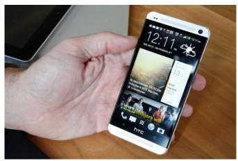
Unibody construction is in aluminium with an optically bonded 4.7-inch LCD display featuring 1920 x 1080 resolution and 468ppi pixel density. Inside are a 1.7Ghz quad-core Snapdragon 600 chip, 2GB RAm, 32 or 64GB of internal storage and a 2300mAh battery. Jelly Bean is the Android version of choice, as reskinned with the latest version of HTC Sense UI.
