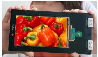
The panel is 1.21mm thick and just 1.2mm at the bezel, making it also the the slimmest and narrowest panel around. Further LG claims include the use of Low Temperature Poly-Silicon (LTPS) substrate for "superior" 430nit brightness with improved transmittance and larger aperture opening size.
