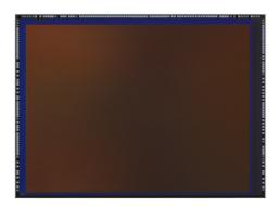
Developed in collaboration with Xiaomi, the sensor promises "extremely sharp photographs rich in detail," even in extreme lighting conditions. It comes in a large 1/1.33-inch size, allowing it to absorb more light in low-lit settings, while pixel-merging Tetracell technology allows the sensor to imitate big-pixel sensor. The result, Samsung says, is brighter 27MP images.
