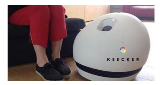
An ex-Google product manager invents the "Robo-Projector." He calls it **Keecker** and it is a rolling robot with a video projector that can sync with smartphones to turn any wall into a screen for watching movies, checking email, and more.
