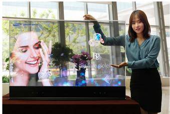
The mirror OLED panel finds use as a "virtual necklace" display at the Chow Sang Sang jewelry company, with the combination of mirror display and 3D cameras allowing customers to play with an interactive (or "self-modelling") wardrobe, with hand gestures providing necessary input. The panel also features higher reflectivity (75%) than similar mirror LCDs, high contrast ratios and no need ambient backlighting.
