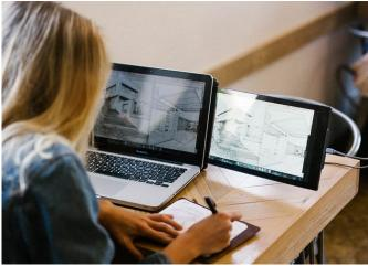
Maker Mobile Pixels says the DUO is a true plug-and-play dual-display laptop solution. It consists of a 12.5-inch 1920 x 1080 resolution IPS display users attach to the lid of the notebook via magnetic mounting system. Once attached, the display slides out from the side whenever required, just like the second display of the 2009 Lenovo ThinkPad W700ds.
