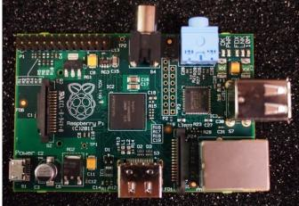
Designed as an affordable PC ideal to get children into computer programming, the Raspberry Pi is a tiny computer the size of a credit card. Currently a simple open board, it carries an ARM processor (running at 700MHz) on top of a Broadcom BCM2835 SoC, together with a Videocore 4 GPU the Foundation says is capable of HD playback.
