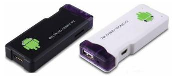
It carries an AllWinner A10 1.5GHz CPU and a Mali 400 GPU supporting 1080p video-out through HDMI port. It uses Android 4.0, but users can also install ARM-compatible Linux versions.
