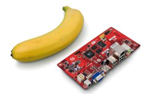
Measuring 17 x 8.5cm, the APC 8750 uses the Neo-ITX form factor and fits in standard Mini-ITX or microATX chasses. It carries an 800MHz VIA WonderMedia ARM SoC (with built-in GPU handling 720p video), 512MB RAM, 2GB storage, x4 USB ports, microSD slot, 10/100 ethernet port and a 15W power adapter.
