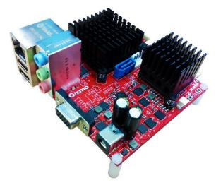
The package includes a dual-core 1GHz G-T40E CPU, Radeon HD 6250 GPU and 1GB of soldered-on RAM, giving it the performance capacity of 52 gigaFLOPS (GFLOPS) according to AMD.
