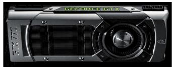
The GTX 770 promises a 5% leap in performance over the GTX 680, but only through slight hops in memory speed (7GB/s vs 6GB/s) and clock speed (1046 vs 1006GHz) paired with an equal amount of CUDA cores (1536).
