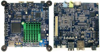
Reportedly the first open source PC with an Intel x86 processor, the Minnowboard development kit is based on Via Technologies processors. The board includes a 1GHz Intel Atom E640 processor, 1GB DDR2 RAM, HDMI port, ethernet, USB ports and microSD slot.
