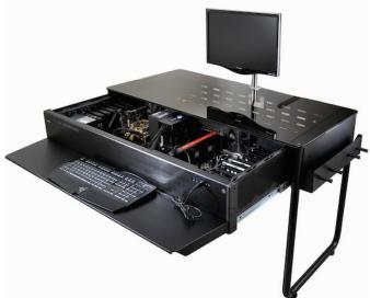
Presented at Computex by Taiwanese case maker Lian Li, the DK-01X and DK-02X are aluminium work desks featuring a lockable sliding drawer with enough space for an HPTX-size motherboard. Or two in case of the DK-02X, since it is large enough to house an extra mini-ITX system.
