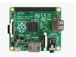
Following the Model B+ upgrade the Raspberry Pi micro PC gets a lower-cost (\$25) variant-the Model A+, a smaller (65mm long) version featuring the same BCM2835 application processor and less power consumption.
