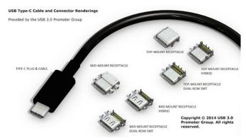
The announcement covers USB Power Delivery (Rev. 2.0, v1.0), USB 3.1 (SuperSpeed USB 10Gbps), and USB Type-C Cable and connector specifications.
