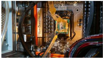
The cooling liquid in question is 3M's Fluorinert FC-72. It acts as an electrical insulator and is colourless, odourless, biologically inert, chemically stable, nonflammable and has a boiling point at 56°C.
