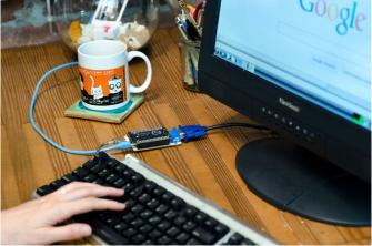
The CHIP features decent enough specs for such a tiny device, with a 1GHz processor, 512MB RAM and 4GB storage. It also carries wifi and Bluetooth radios, micro USB port, composite video-out (can be turned into a VGA or HDMI port via optional adapters) and integrated battery power circuit, all within open source hardware.
