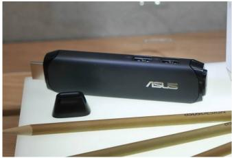
Similar in size and shape to an oversized USB flash drive, the Pen Stick connects to displays via HDMI connector. It features two USB 2.0 ports, micro USB 2.0 port (handles power duties), microSD reader, combo audio jack and wireless connectivity via 802.11b/g/n wifi and Bluetooth 4.0.
