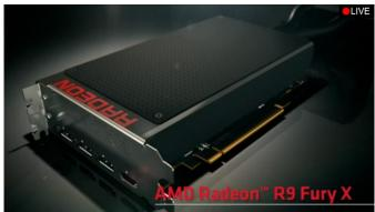
Based on the "Fiji" chip, the R9 Fury X has "the highest GPU memory bandwidth ever" through the use of <a href="high-bandwidth memory">high-bandwidth memory</a> (HBM), a GDDR5 RAM replacement consisting of vertical memory stacks. This allows for more memory within less board real estate, as well as for smaller graphics cards.
