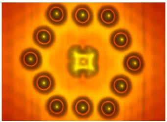
For the curious, the team used a highly stable scanning tunneling microscope (STM) to build the transistor out of a single molecule of phthalcocyanine and 12 positively charged indium atoms on an indium arsenide (InAs) crystal. The indium atoms act as electrical gates, allowing single atoms to hop over to change the charge state of the molecule.
