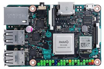
Officially dubbed the "Asus 90MB0QY1-M0EAY0," the Tinker Board measures 8.5 x 5.3cm and carries a quad-core 1.8GHz ARM Cortex A17 CPU, ARM Mali-T764 GPU and 2GB DDR3 RAM. The combination, according to the company, allows 4K video and 24-bit audio support through H.265 4K decoding, and should also allow for better 3D graphics performance.
